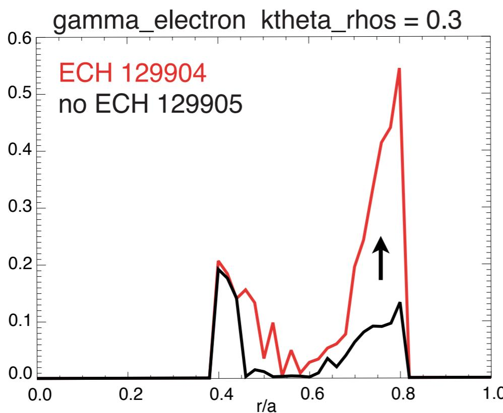
Growth rate of electron mode at fixed  $k_{\theta} \rho_s = 0.3$  increases across the radius, but largest increase at  $\rho \sim 0.75$
