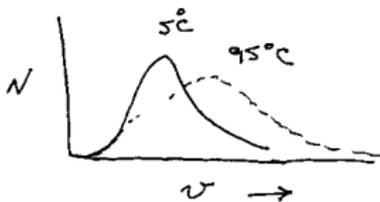
High energy particles will exchange energy of lower energy particles
