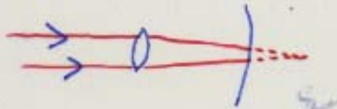
Eye can accommodate diverging rays but only up to a near point  $> 25\text{cm}$
