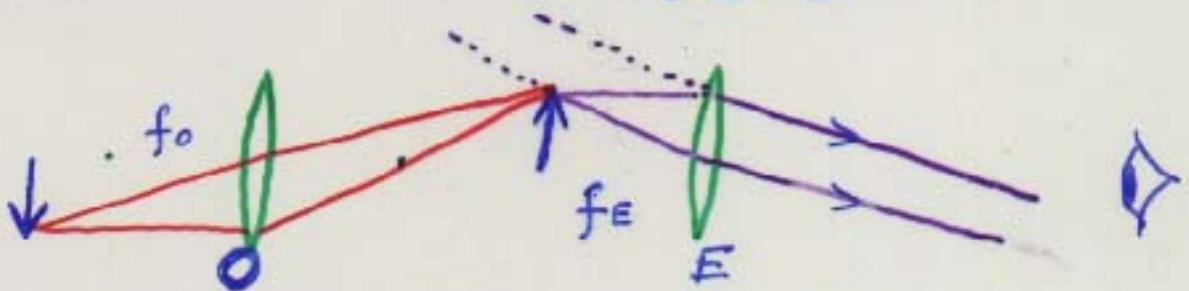
Intermediate image placed at focus  $f_E$  of eyepiece.
