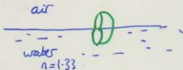
split lens to focus above/below water simultaneously
