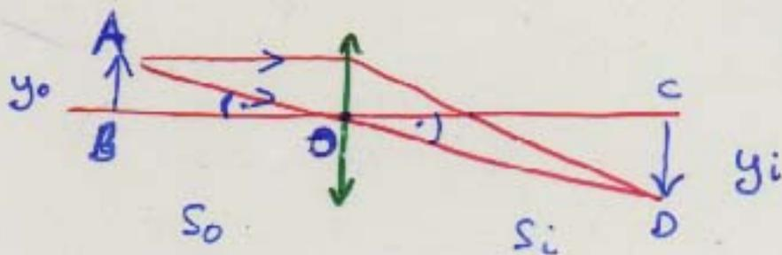
In dimension  $\perp$  to optical axis, image can be magnified ( $y_i > y_0$ ) or minified ( $y_i < y_0$ )
