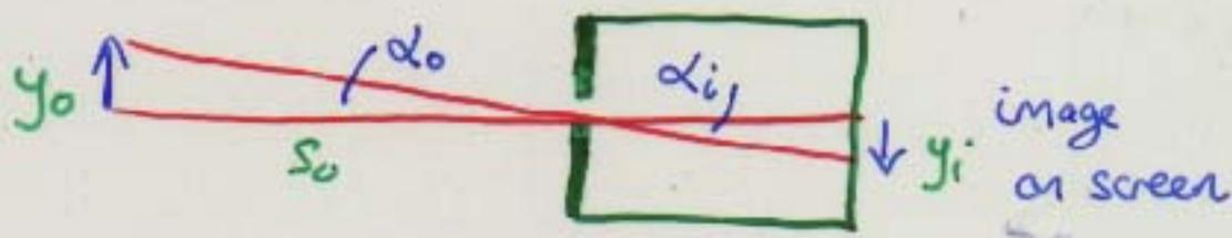
Magnification  $y_i/y_0$  depends on hole-screen distance  $s_i$ .
