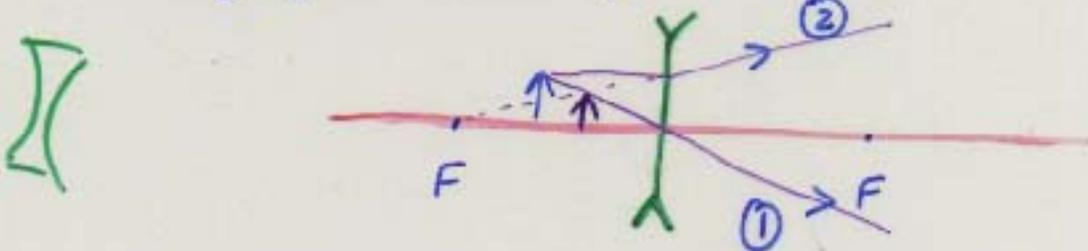
If  $s_o = 3\text{cm}$ , image is virtual, erect, magnified
