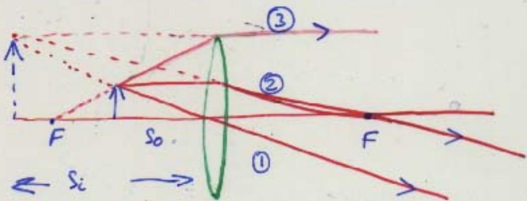
image is virtual, erect, Magnified
