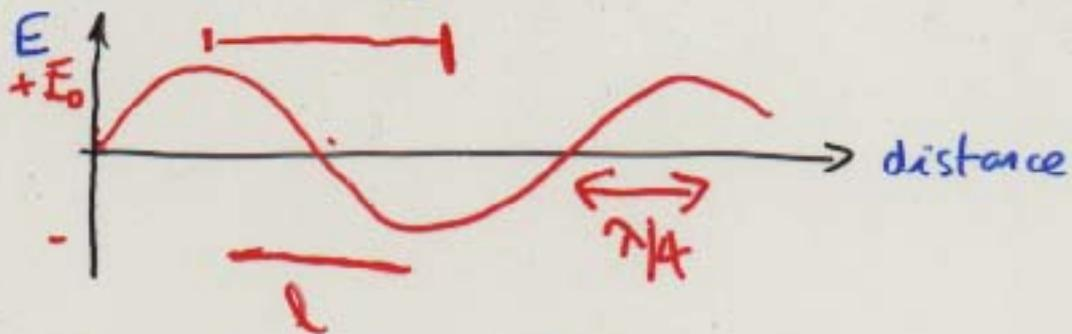
For wire placed along EM wave, max. difference in  $E$  between ends is when length  $l = \lambda/4$
