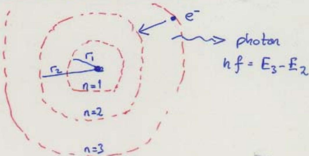
Quantized orbits: can explain spectral line wavelengths
