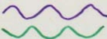
As long as sources are coherent (same offset in phase over time), interference pattern is stationary (i.e. can be observed)
